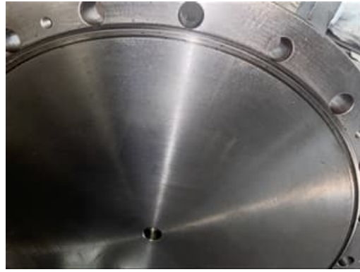
The lower outer manhole (1)
