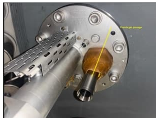
Premix gas passage burner #12
