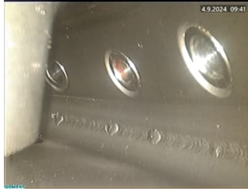
Burner #10 inner chanel with droplets of water
